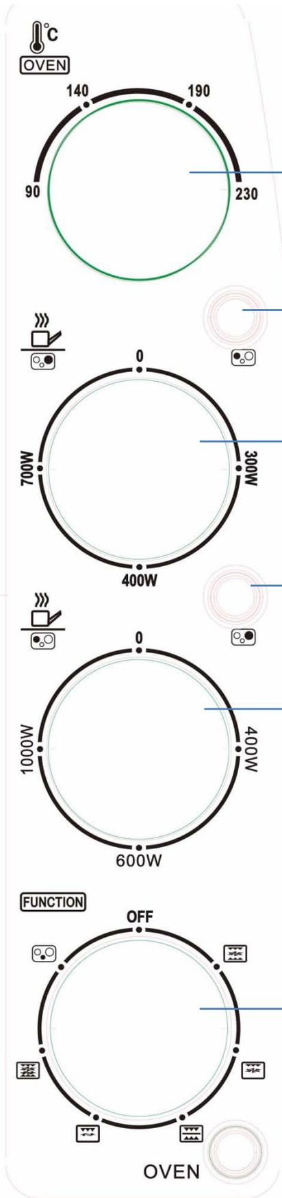
**Temperature Knob:** the temperature choice is from 90 to 230°C. You could select desired temperature according to the practical use
